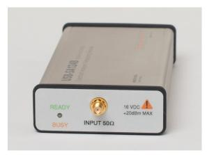
The **front panel** includes a  $50\Omega$  SMA RF input. Do not exceed +20 dBm or +16VDC or damage may occur. A **READY / BUSY** LED flashes orange each time a command from the computer is processed.
