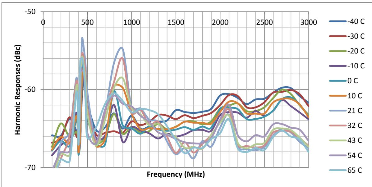
\*Signal 10 dB below reference level. To calculate IP2 at a given frequency, subtract this number from signal level (e.g. -30 dBm reference level would be a -40 dBm signal. Subtract e.g. -64dB @ 2 GHz for an IP2 of +24 dBm).
